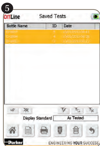
5 Export results: Highlight the test result(s) you would like to export using the stylus.
